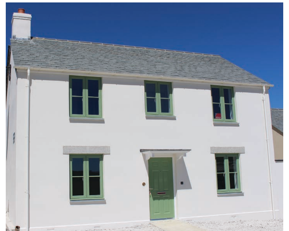
Granite is used for lintels and landscaping. Slate is used for cills and roofs.
